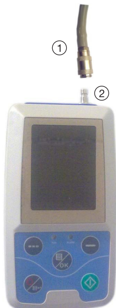
Figure 1 The top external airway
